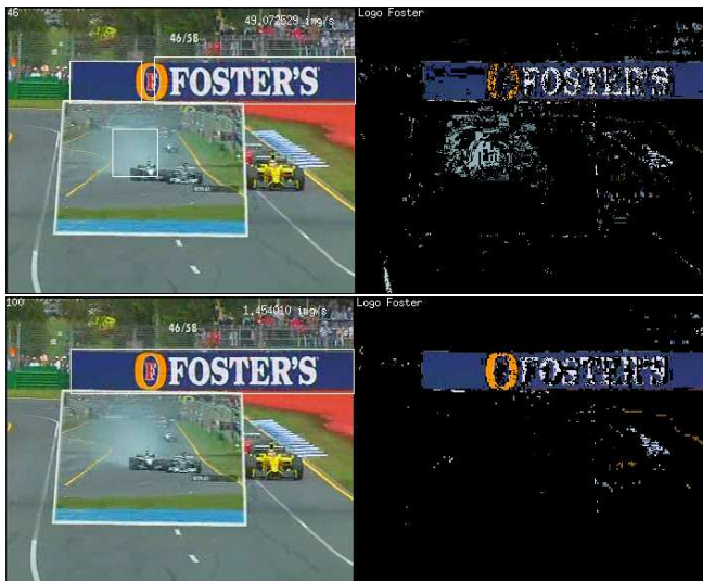
Fig. 4 Detection using chrominance (top) vs detection using receptive fields (bottom)
