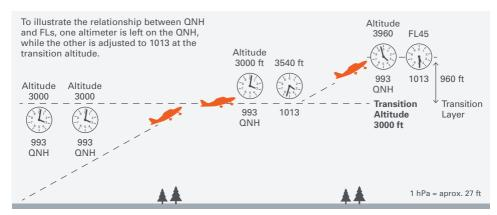
On this day the QNH is 993 hPa. When the aircraft reaches the transition altitude (3000 ft AMSL in this example) and 1013 hPa is set, the altimeter will read 3540 ft. Assuming the aircraft is traveling westbound, the lowest available VFR FL is 45.
