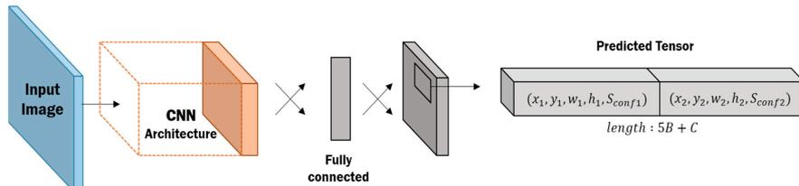
**Fig. 10.** Yolo uses a CNN architecture followed by a fully connected layer to simultaneously bounding boxes and classes for objects. Image copied from [13].
