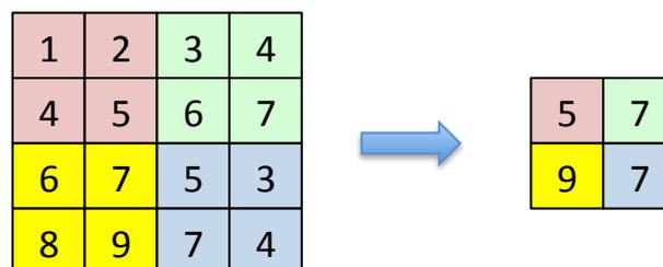
**Fig 6.** Max pooling replaces an  $N \times N$  window of features with the largest feature value in the window. For example the  $2 \times 2$  red square in the upper left corner is replaced by the largest of the 4 values in the square (5).
