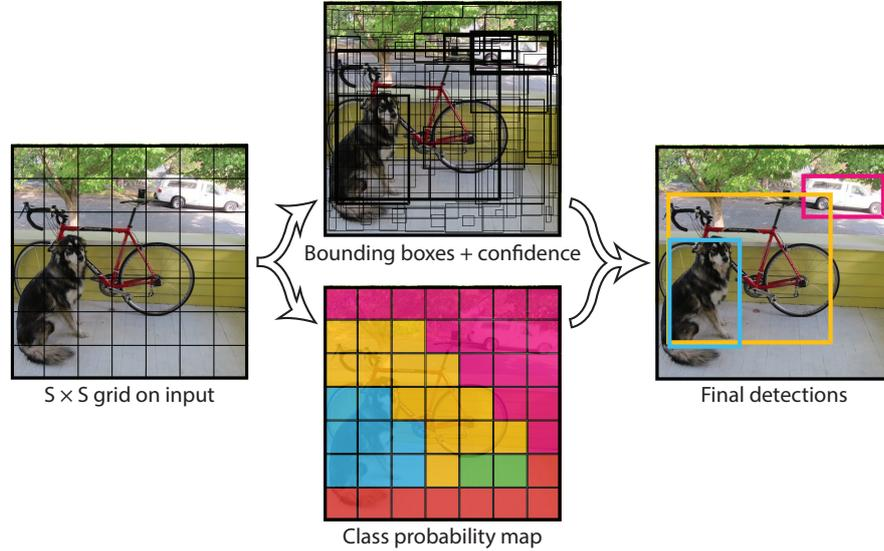
**Fig 9.** You Only Look Once (YOLO). The Yolo network simultaneously estimate bounding box coordinates and class probabilities for objects. Image copied from [12].
