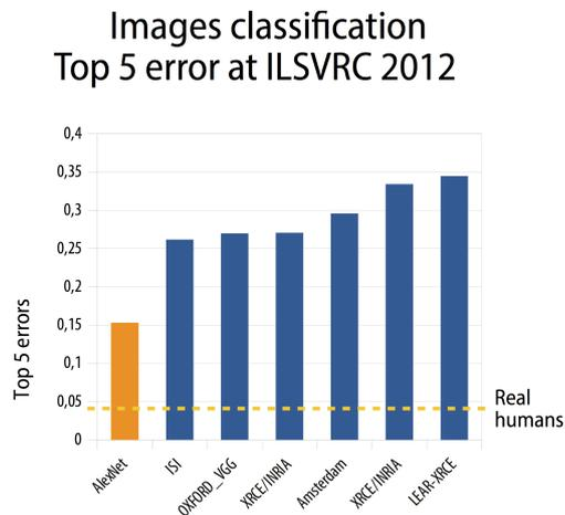
**Fig 7.** Error rates for the top 5 entries in the 2012 ImageNet Large Scale Visual Recognition Challenge (ILSVRC) [9]
