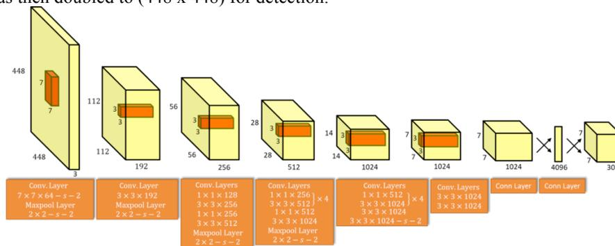
Fig 11. YOLO is composed of 24 convolutional layers followed by 2 fully connected layers. (from: <http://datahacker.rs/how-to-peform-yolo-object-detection-using-keras/>)
