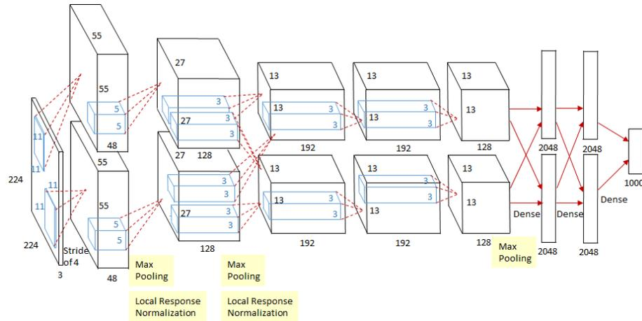
**Fig. 7.** The AlexNet architecture [10].
