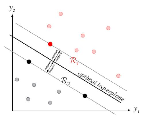
**FIGURE 5.19.** Training a support vector machine consists of finding the optimal hyperplane, that is, the one with the maximum distance from the nearest training patterns. The support vectors are those (nearest) patterns, a distance *b* from the hyperplane. The three support vectors are shown as solid dots. From: Richard O. Duda, Peter E. Hart, and David G. Stork, *Pattern Classification*. Copyright © 2001 by John Wiley & Sons, Inc.
