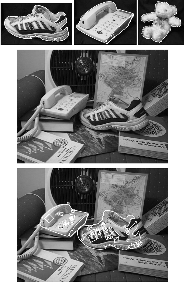
Figure 4: Top row shows model images for 3D objects with outlines found by background segmentation. Bottom image shows recognition results for 3D objects with model outlines and image keys used for matching.
