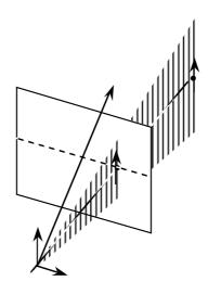
The equation  $M_s^1 \cdot R_k^s - i_k (M_s^3 \cdot R_k^s) = 0$  is the vertical plane that includes the projective center through the pixel  $i=i_k$ .
