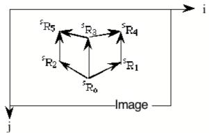
The matrice  $M_s^i$  is composed of 3x4=12 coefficients. However because,  $M_s^i$  is in homogeneous coordinates, the coordinate  $m_{34}$  can be set to 1.
