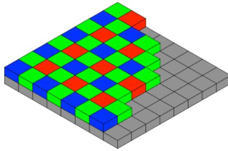
The voltage values on each sensel are converted to numeric values, interpolated and processed to provide image pixels. This step is sometimes called “image reconstruction” in the image processing community, and is generally carried out on the retina. The result is generally an image with colors coded as independent components: RGB.
