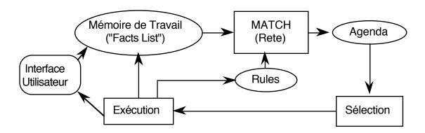
The system implements an "inference engine" that operates as a 3 phase cycle:
