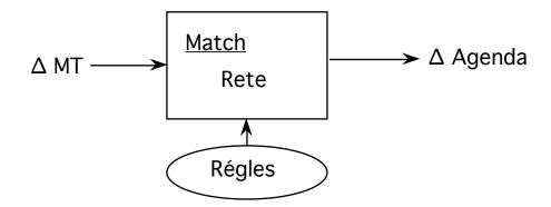
RETE is an incremental matching algorithm. The word RETE is Latin for "network". RETE operates by compiling the rules into a decision network.
