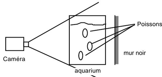
4) You are asked to design a system to detect and follow tropical fish in an aquarium. The Aquarium is well illuminated by several spotlights with a white spectrum. The back wall of the aquarium is matte black. A color camera is placed such that the aquarium is entirely within the visual field of the camera. The fish have unique colors. You are requested to estimate the position of each fish in each image.
