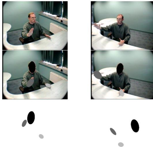
**Figure 1.** Left: left and right captured images. Center: left and right images with projected ellipsoids. Top right: ellipsoids projection on the frontal plane. Down right: ellipsoids projection on the side plane (the cameras are on the left side).
