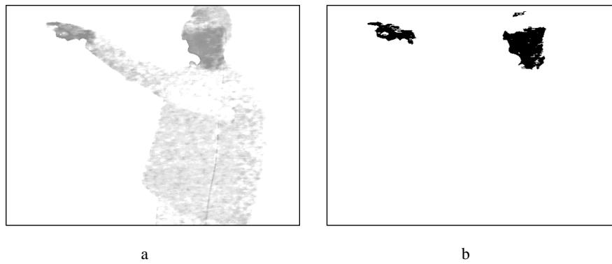
**Fig. 4.** a) Red channel of the pre-segmented camera image. b) Thresholded red channel after labelling the three largest objects. The gray values of the images are inverted for representation purpose.
