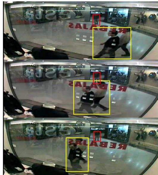
**Figure 3** Tracking module with Kalman filter and shape extraction and association is able to maintain objects identities during occlusions
