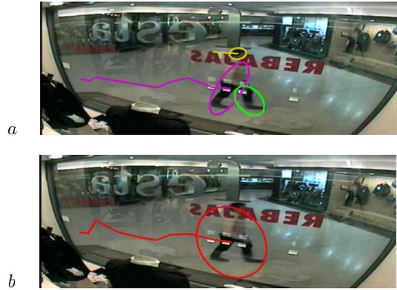
**Figure 1. a: 3 clusters tracked by the cluster tracker at frame 90, test sequence 1. b: the 3 clusters are grouped into a single super-cluster during post-processing.**
